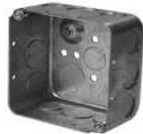
4" square deep steel box* 4" x 4" x 2-1/8" (102mm x 102mm x 54mm)
